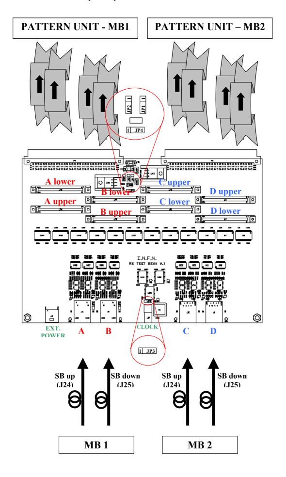
Example setup for MB1 and MB2 chambers
