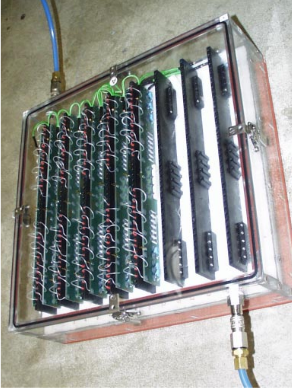
HV board final test jig (under proper gas)
